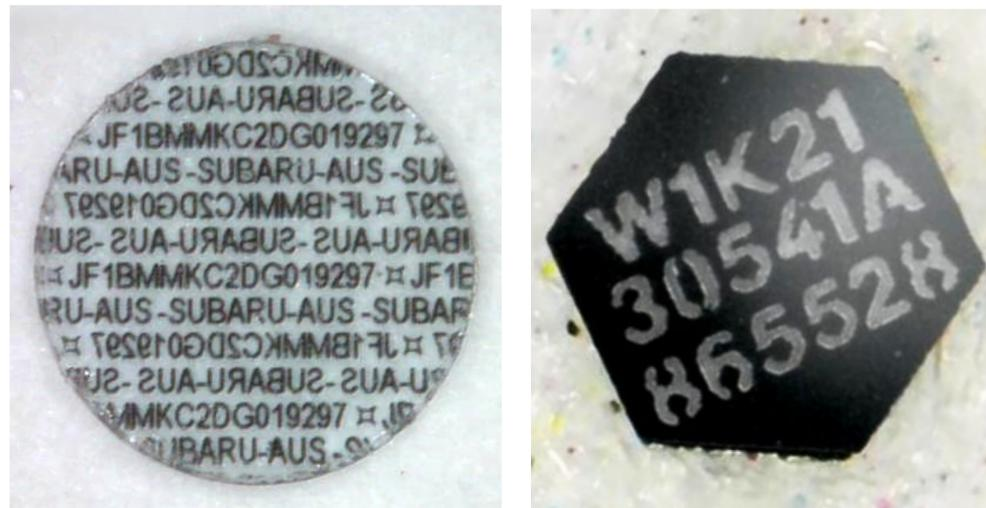
Examples of 2 types of microdots, both showing a 17 character motor vehicle VIN
