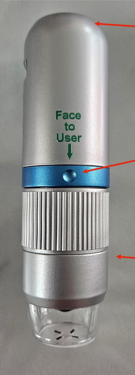
Change the brightness of the reader's lamp by turning the knurled wheel on top of the reader.
